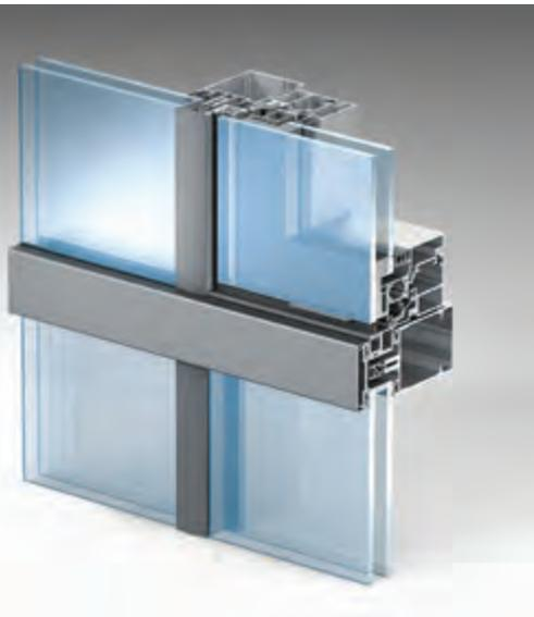
In this facade modification, a vertical or a horizontal line is outlined with the help of various massive clamping bars (oval, hemispheric or rectangular), therefore adding some horizontal or vertical volume. Along other lines the clamping bars are replaced by seam sealing or the space between the IGUs is filled up by silicon seam sealant.
