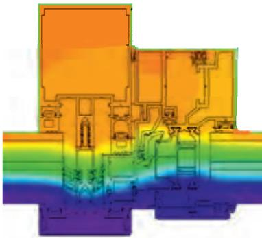
1 3/8" (34 mm) polyamide thermal breaks help to keep the thermal conductivity of the frame-sash section at  $U_f = 1,9-1,7 \text{ W/m}^2\text{K}$  which is much better than the indexes of European equivalents within facade windows segment.
