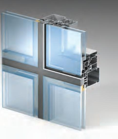
This system allows fabrication of all-glass look facades of any configuration without aluminum profiles on the outside surface. Insulated glass is fixed to mullions with hidden clamps.
