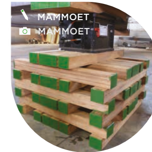
Mammoet Jacking Beams The Netherlands
