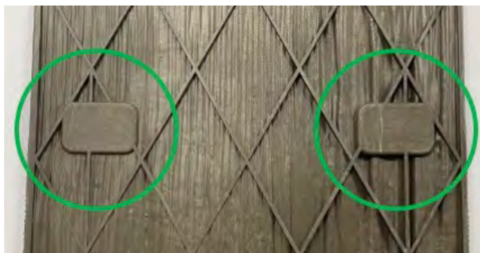
Figure 2.7.3 Fastener pads (back)
