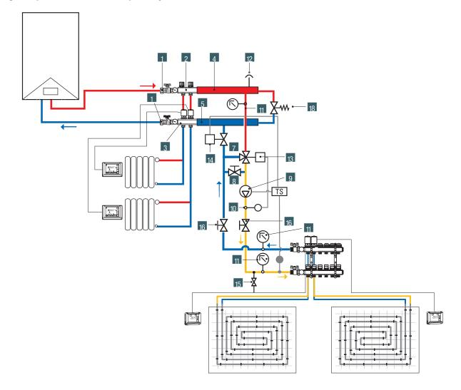
Hydraulic scheme - distribution system for low-temperature heating systems with auxiliary connections for high-temperature terminal. Climatic regulation.
