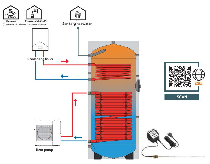
The HP2V series storage tanks are suitable for the production of domestic hot water using a heat pump and boiler. They are supplied with the closing flange mounted and provided with thermal insulation and nr. 1 electronic anode.
