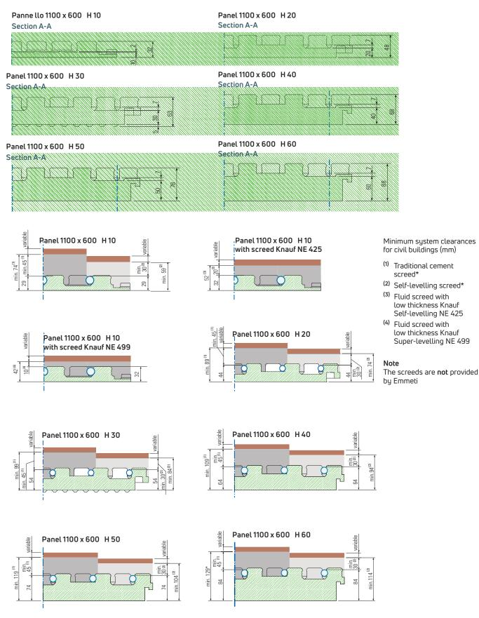
The effective thickness of the screed and the mode of construction of the same are to be defined with the manufacturer / supplier of the same according to its specifications, depending on the conditions of installation (size and type of installation surface, type floor, etc.) and of the type of slab chosen.
