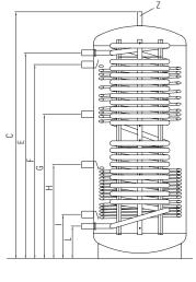
EB1000-1500 storage tanks are designed to be able to integrate multiple energy sources present in the heating system, such as, for example: heat pumps, thermal solar panels, gas boilers, thermo fireplaces, etc.
