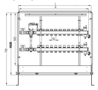
Combination of Topway 1" manifolds in metal cabinet
