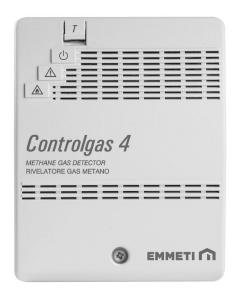
Methane gas leak detector for domestic use with the possibility of directly controlling a 230 Vac solenoid valve. Equipped with test button.
