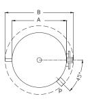
HYBV1S series storage tanks consist of a double storage tank for the production of domestic hot water from a heat pump with thermal flywheel for hot or chilled technical water.
