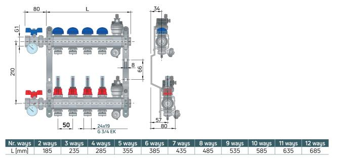
Topway S distribution manifold in stainless steel, with lockshields with flow meters included
