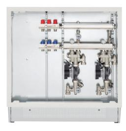
Distribution modules for low-temperature heating systems with mixing valve, auxiliary connections 2 or 3 high temperature radiators, electronic circulation pumps.
