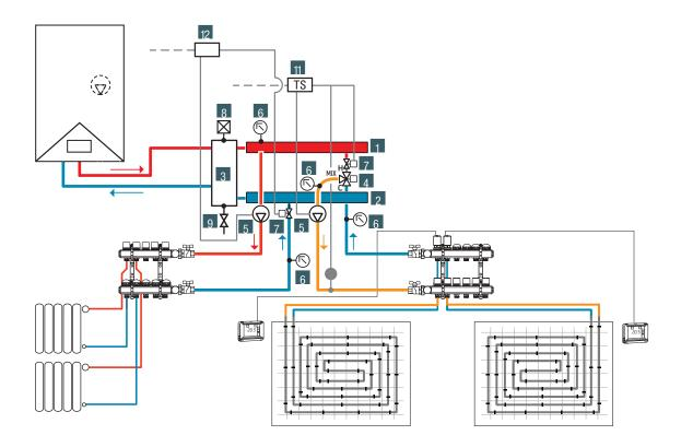
Hydraulic scheme - Modules for low temperature heating systems with auxiliary connections for high temperature terminals. Thermostic regulation
