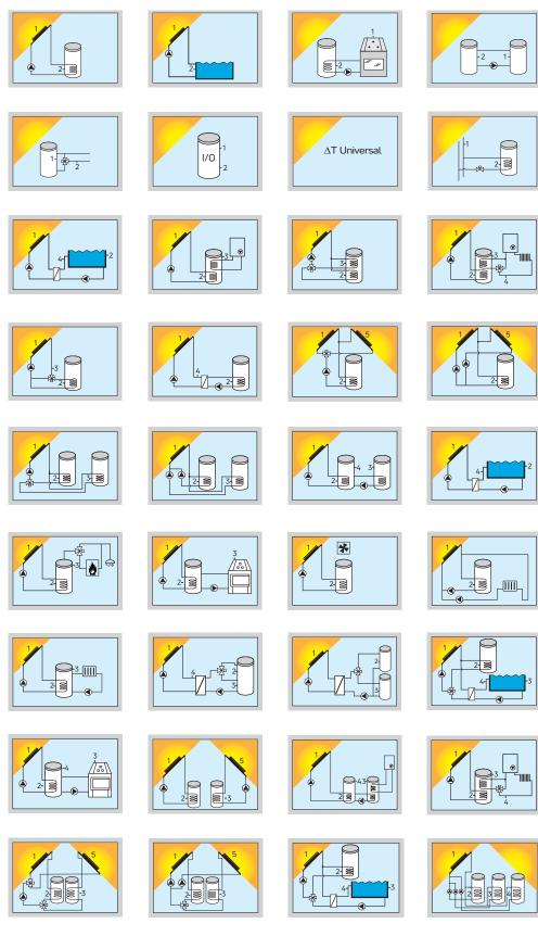
Basic hydraulic variants with ELCS 2016 differential temperature controller and SSC40 NP solar station
