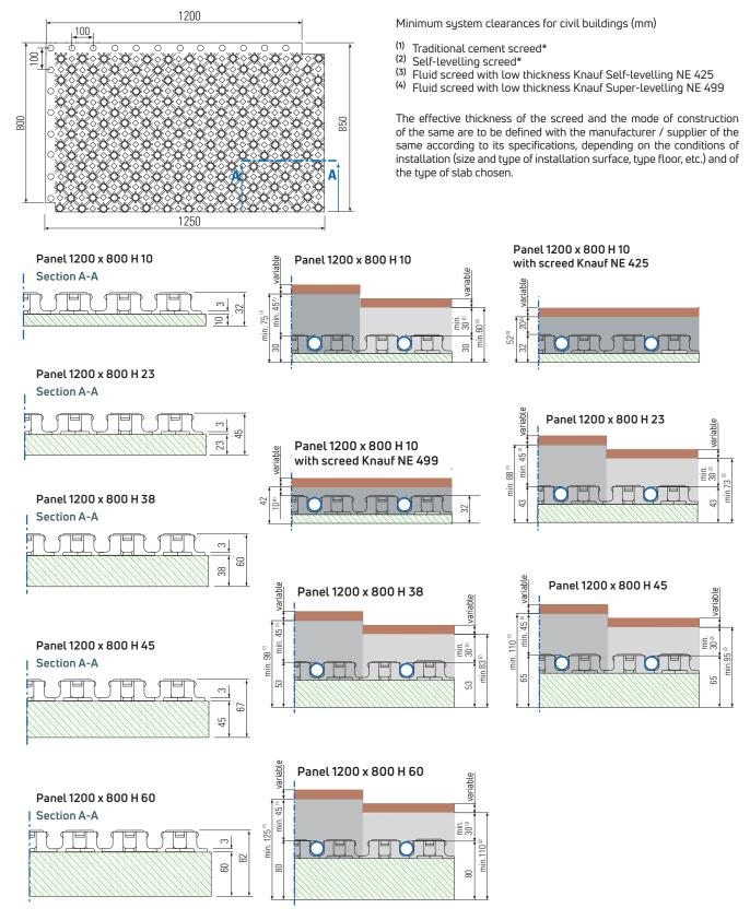
\* If the Emmeti Floor system is combined with the Mirai SMI + Febos 4.0 heat pump, it is advisable to increase the thickness of the screed by about 1 cm from the minimum values.
