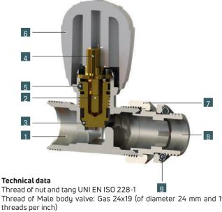
Thread of Male body valve: Gas 24x19 (of diameter 24 mm and 19 threads per inch) Thread fo Female body valve UNI EN ISO 228-1 Maximum operating pressure: 10 bar Maximum differential pressure: 1 bar Maximum operating temperature: +100 °C Large capacity Fitting also available with O-ring (NBR)
