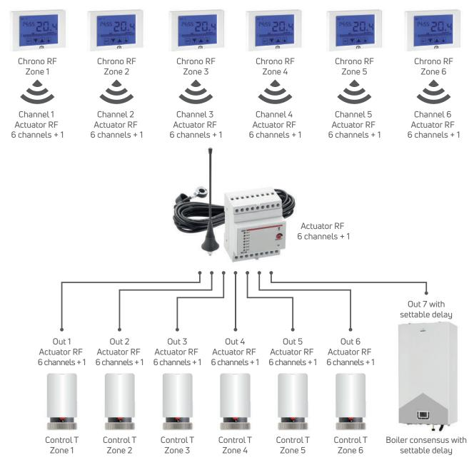
Use: autonomous multi-zone system (up to 6 zones) where the zones can be intercepted in a single point, for example with electrothermic heads installed on a manifold
