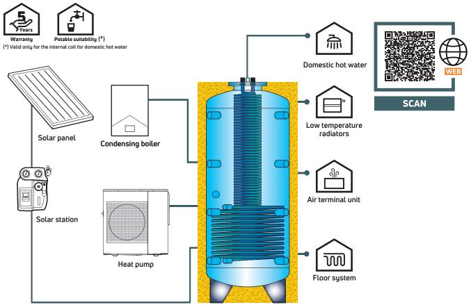
EBN300-500 and EB1000-1500 tanks have been designed to integrate more energy sources existing in the heating system, for example: heat pumps, solar panels, gas boiler, thermo fireplaces, etc.
