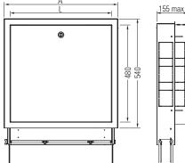
Metalbox for 80 and 120 mm brick thickness (frontal ways body + frame + door)
