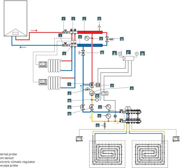
A external probe B room sensor C electronic climatic regulator D flow pipe probe
