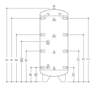
Puffer are used for the storage of heating water in support of systems with boiler, wood-burning boiler, thermal stove, fireplaces and other sources of energy.
