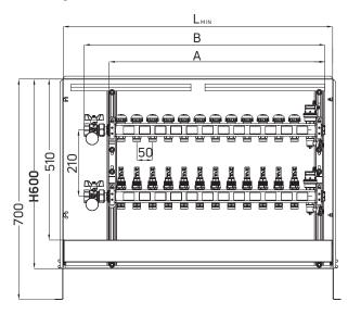
In combination with Topway S manifolds in metal cabinet
