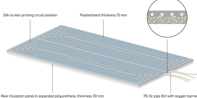
PE-Xc pipe 8x1 with oxygen barrier
