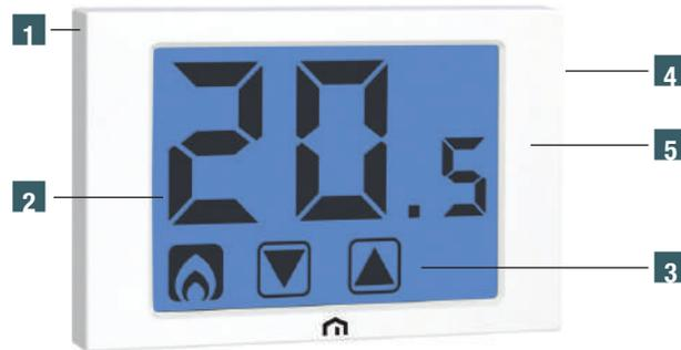
Electronic thermostat with backlit touch screen with wall installation, designed for room temperature control both in heating mode (winter) and in air conditioning mode (summer). The keyboard consists of two icons located in the lower part of the touch screen display. Available in mains or battery powered versions.
