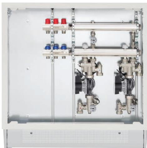
**Distribution modules for low-temperature heating systems with mixing valve, auxiliary connections 2 or 3 high temperature radiators, electronic circulation pumps.**
