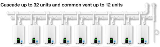
With Navien cascading technology, when a unit gets up to 80% capacity the next unit will turn on to help meet requirements. This demand ratio will continue until all 32 units are generating hot water. The Navien cascading system also balances out the workload of each unit for longer life. Building penetrations are reduced with Navien's common venting feature.
