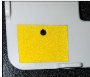
The mounting bracket has a reflective corner that must be lined up with the infrared detection sensor. If performing bench testing, then it's recommended to turn off Tamper detection, as this will impede testing performance if the Infrared sensor is not properly lined up with reflective surface. Please see "*Beep/Flash indication - Switch #1 Group Settings*" section for more details on how to adjust Tamper Sensor settings.
