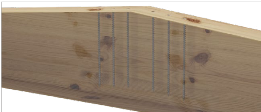
Reinforcement with screws in roof ridge area
