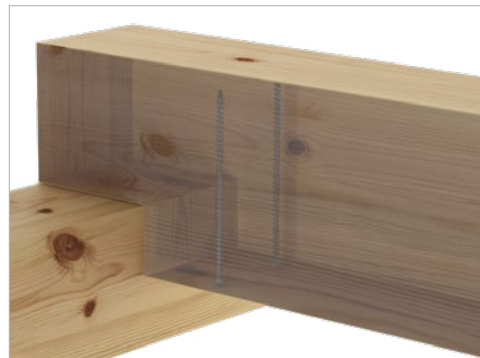
Protection against failure of notched beam
