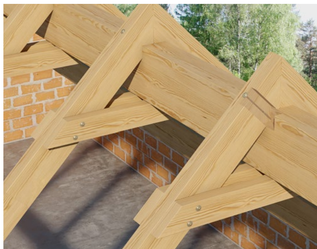
Construction of roof truss
