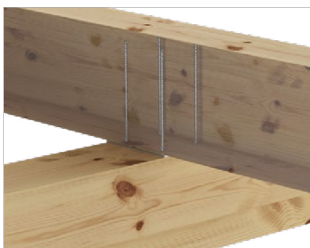
Reinforcement in the point of support
