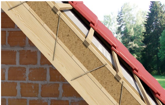
Fixing of soft over-rafter insulation Insulation material with a low compressive strength ( \sigma(10\%) < 50 \text{ kPa} - EN 826)
