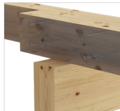
Joint between two passing-by beams
