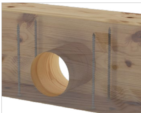
Reinforcement of beam in the point weakened by drill hole
