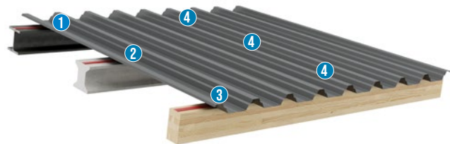
Fig. 2 - Flat roof without thermal insulation
