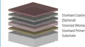
Stontec TRF is a urethane flake floor system designed for maximum durability and impact resistance.
