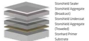
Stonshield HRI is a textured system that cures to an extremely hard, high impact-resistant surface which is decorative and exhibits excellent abrasion, chemical and High-Impact resistance.
