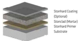
Stonclad HT cures to an extremely hard, impact-resistant mortar which exhibits excellent abrasion, wear resistance and superior chemical resistance. It can be used anywhere chemical-resistant epoxy mortar is required.
