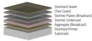
Stontec UTF is a urethane-based system that combines a decorative appearance with chemical, stain and wear resistance. This system creates a stain-resistant surface that can be installed quickly with little odour.
