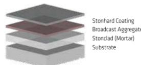
Stonclad UT provides the added texture that is required in many pharmaceutical companies. Due to its resistance to harsh and continuous chemical attack, impact and abrasion, Stonclad UT has the ability to stand up to thermal cycling and thermal shock.
