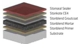
Stonblend HDF is a decorative epoxy mortar system suitable for heavy duty environments.
