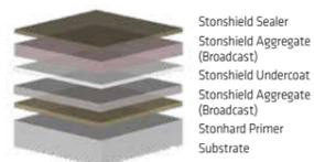
Stonshield SLT is a cost-effective, textured, decorative epoxy system with reduced resistance to heavy impact and loads. Ideal for light manufacturing and commercial environments.
