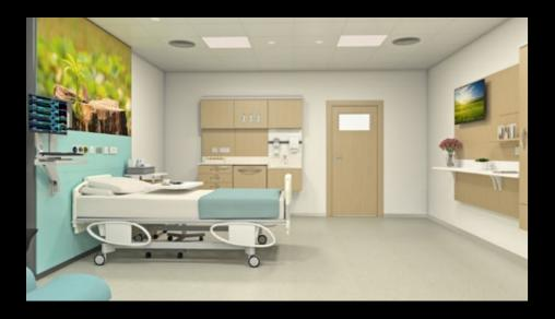
Thanks to String<sup>2</sup>'s versatility, functionality and its many combination and integration options, this innovative wall system is in demand for healthcare applications. The steel walls score high in terms of hygiene, fire resistance, air tightness, durability and acoustic properties. They are also X-ray proof and can be provided with antibacterial coatings.
