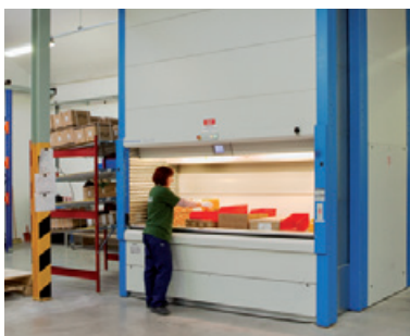
Kardex: automated high-capacity storage system.
