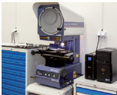
Profile projector at the Quality Management Laboratory.
