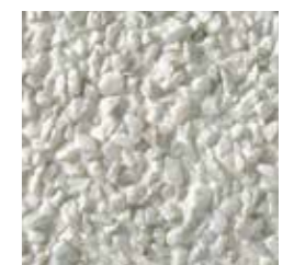
C: Coarse [5-8 mm] Thickness: 14.0 ± 0.6 mm
