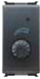
GW 30 403 ▲ Resistive 230 V ac 100-900 W Resistive 110 V ac 100-500 W Inductive 230 V ac 40-300 VA Inductive 110 V ac 20-150 VA GW 30 404 Resistive 230V ac 40-300W Resistive 110V ac 20-150W Inductive 230V ac 40-300VA Inductive 110V ac 20-150VA With two-way switch
