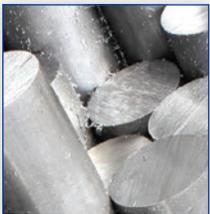
Ultra's high strength, aluminum alloy is as strong as steel, but will never rust. Our 6005-T5 alloy has a minimum strength of 35,000 psi.
