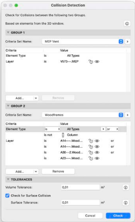
Collision detected between wood construction and MEP element
