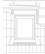
recessed installation - concrete roof
