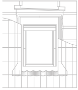
recessed installation above rafter insulation
