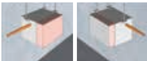
An RB unit can be installed on either side of the control box.
