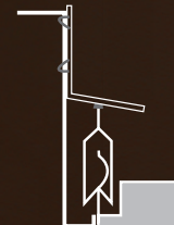
Snap "T" with adjustable side supports
