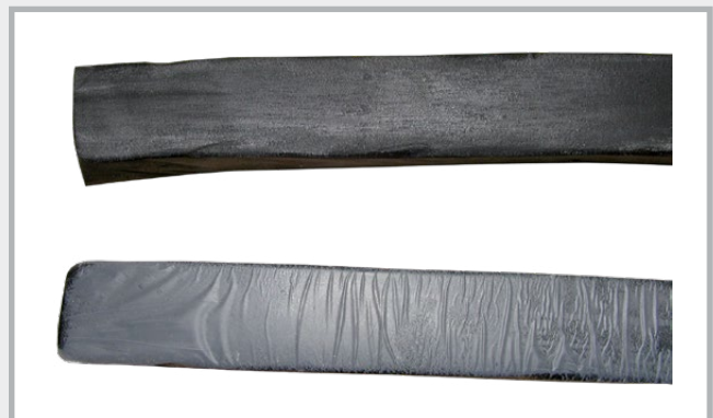
Comparison of swelling tape with and without protective film
