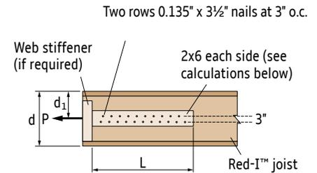
To calculate the length of the filler block (to transfer shear to joist flange):
