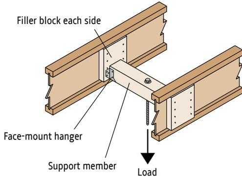
Each side of the bottom flange of the Red-I™ joist can support a 250 lb maximum load at 5' on-center (provided the load is included in normal design loads). Use detail 9 above for loads exceeding this limit.
