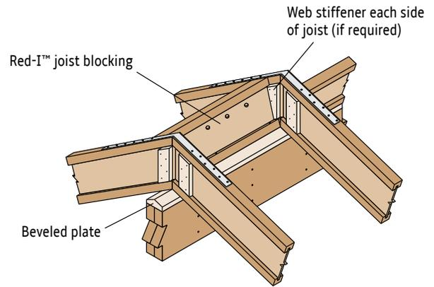
*A strap and alternating blocking panels, or two rows of blocking panels, are required for lateral stability.*
