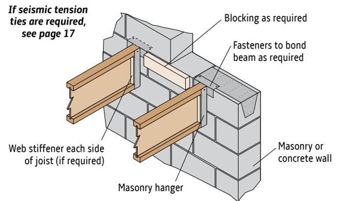
*Traditional masonry hangers will not support construction loads without a minimum amount of cured masonry construction above hanger level. Refer to hanger manufacturer's literature for information on the correct installation and use of masonry hangers.*
