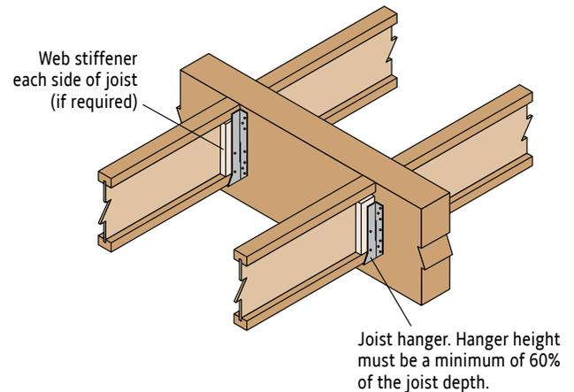
*Web stiffeners are required if the sides of the hanger do not laterally support at least ¾" of the Red-I™ joist top flange.*
