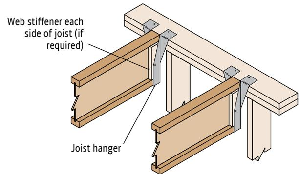
*The potential for top plate rotation may reduce hanger capacities. Contact RedBuilt for assistance.*
